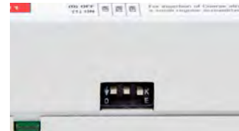
Side-mounted DIP switches let you switch between modes before installation.
