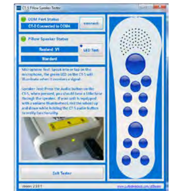
The included software shows which pillow speaker functions are being tested
